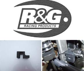
• Fit the mounting bracket (see picture above) to the frame using the M8x20mm long cap head bolt, with a 8mm washer under the head of the bolt.
